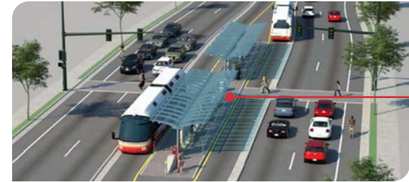
Median-Running BRT Station @ Mid-Block
